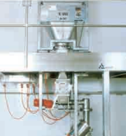
Feeding and sifting station for Pharmaceutical powders
