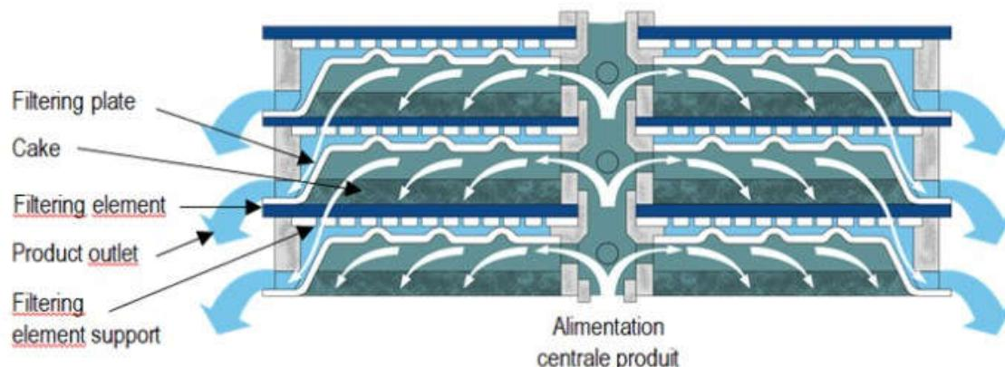
The horizontal arrangement of plates facilitates uniform distribution of solids on the entire filtering area and good stability of the obtained cake.
