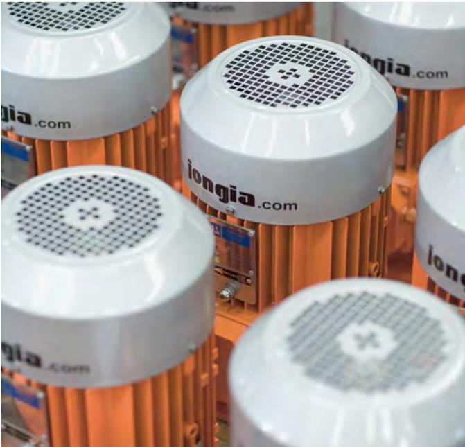
With a maximum installed power of 11 kW and longest shaft extensions of approx. 10 metres, JDR mixers' construction requires a minimum of headroom thanks to its low height and the noise levels produced by these mixers are extremely low. A pole reversible motor is available as an option, allowing the mixer to run at two different speeds.
